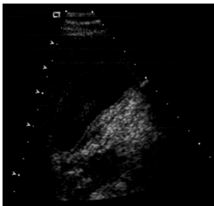
image too dark—first, increase receiver gain
